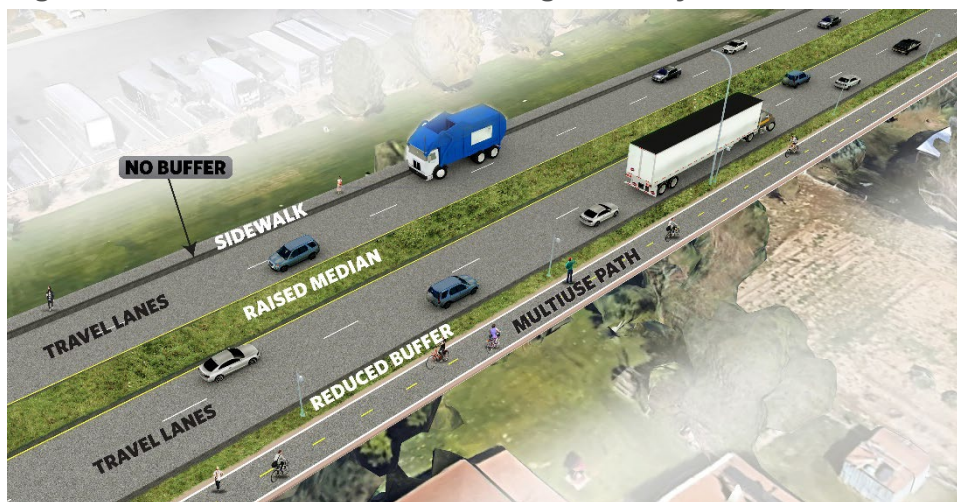
Figure 8. Minor Arterial—95-Foot Right-of-Way
