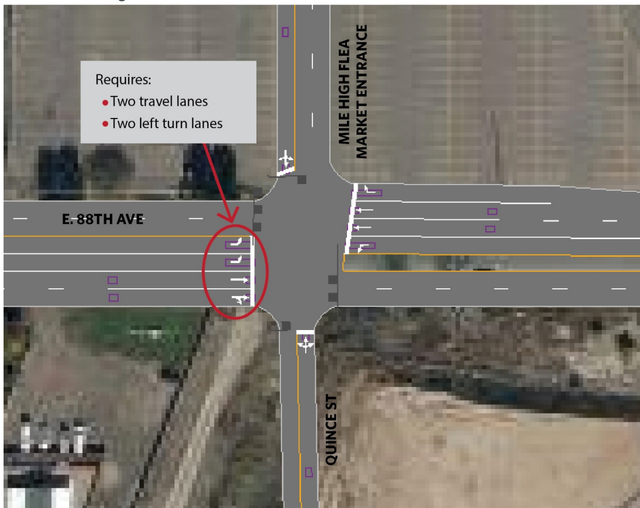
Figure 17. North Side Access Option 1: Double Eastbound to Northbound Left-turn Lanes to Mile High Flea Market
