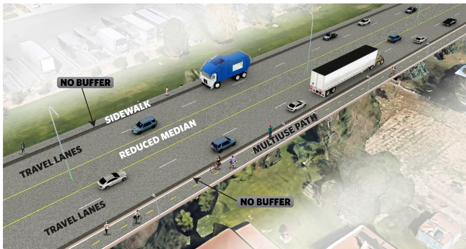
Figure 9. Minor Arterial—82-Foot Right-of-Way
