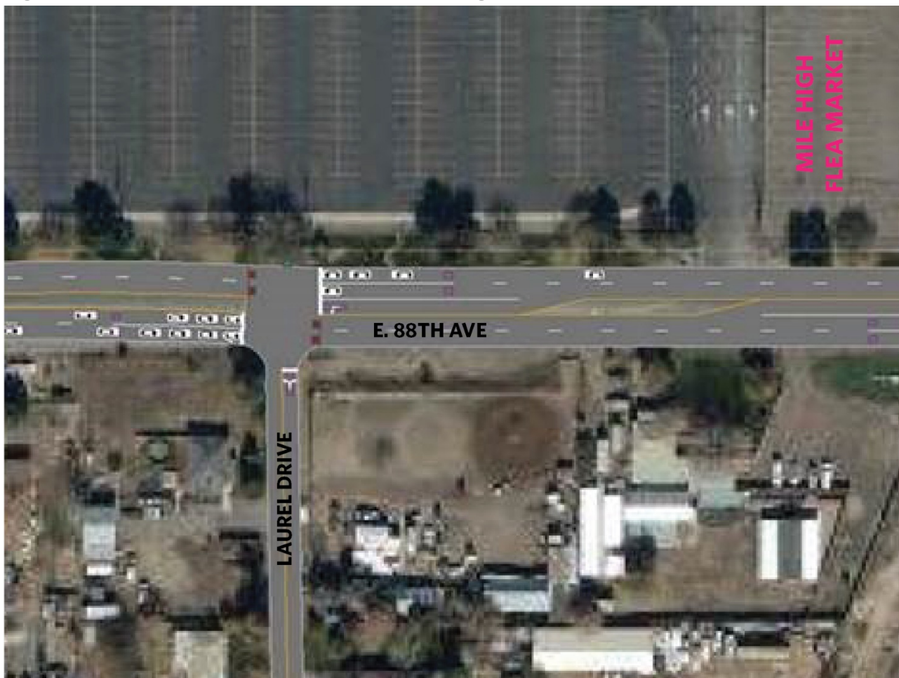
Figure 15. South Side Access Option 3: New Signalized Intersection at Laurel Drive
