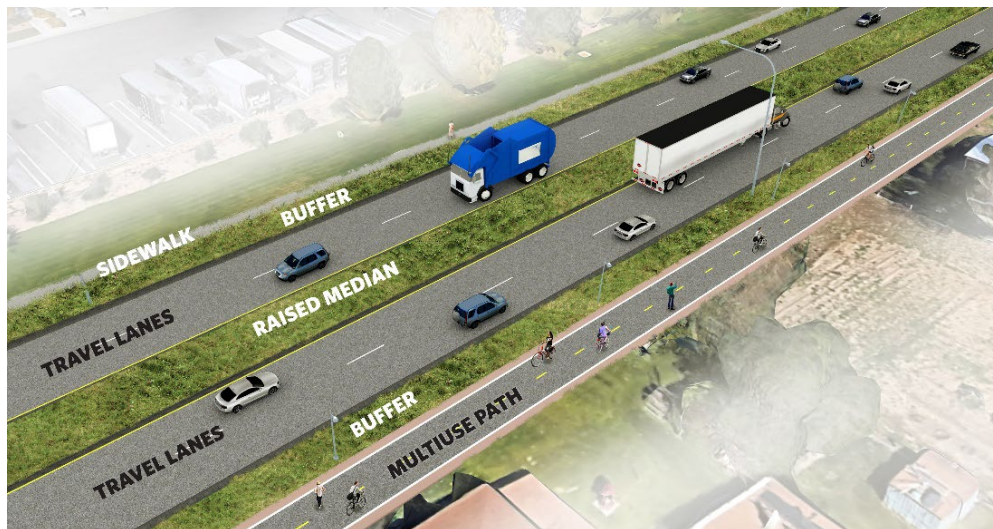
Figure 7. Minor Arterial—120-Foot Right-of-Way
