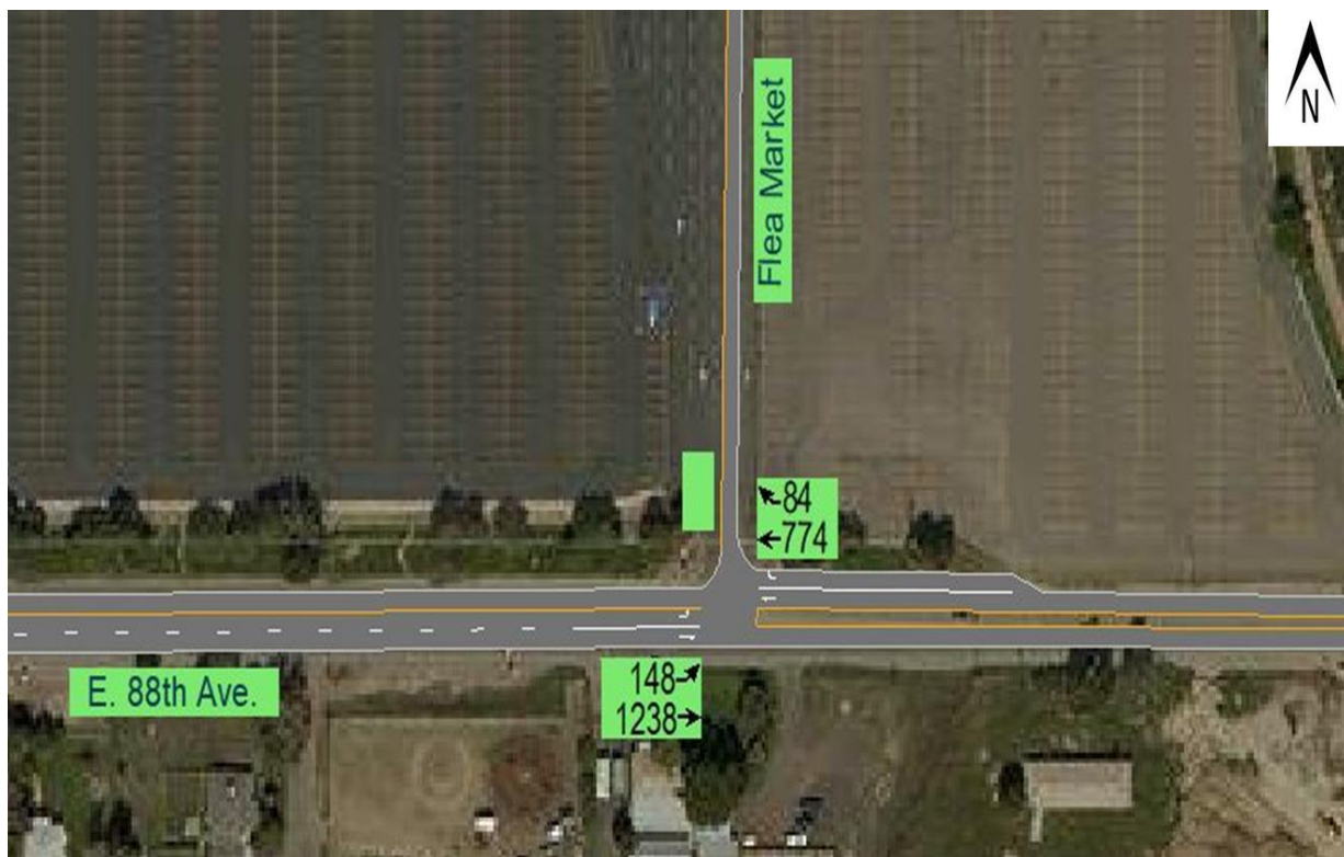
Figure 8. Traffic Volumes Estimated on Friday at Mile High Flea Market Entrance in 2019 - Synchro 10 Graphic
