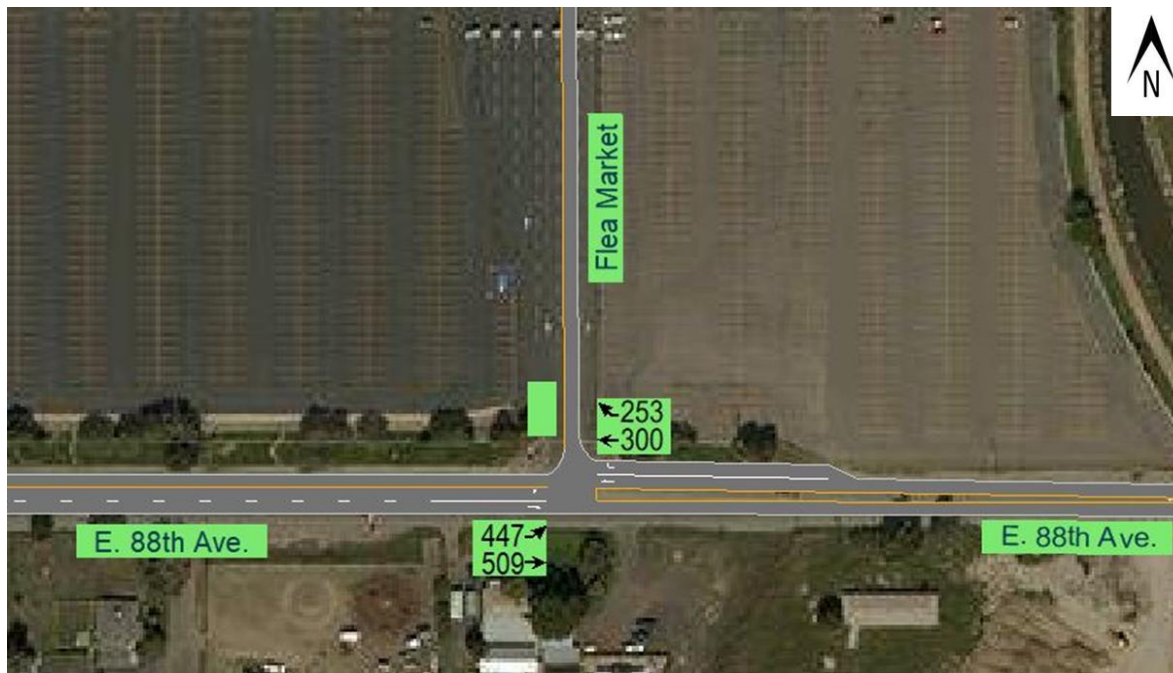
Figure 7. Traffic Volumes Estimated on a Sunday at the Mile-High Flea Market Entrance in 2019 – Synchro 10 Graphic
