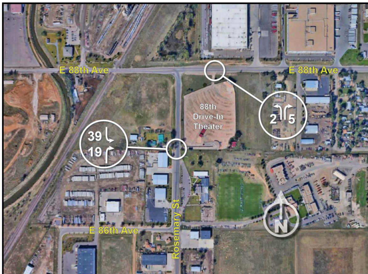
Figure 9. September 2019 Traffic Counts Collected on Friday 4:00 PM to 6:00 PM at 88 Drive-In Theatre
